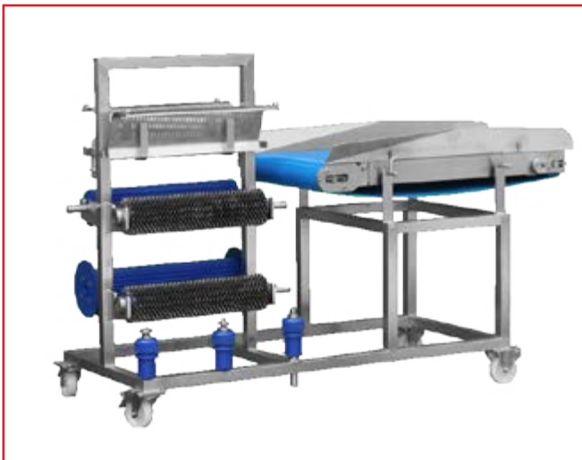
The tool rack accessory can hold extra rollers, guides, and belt for sanitation.
