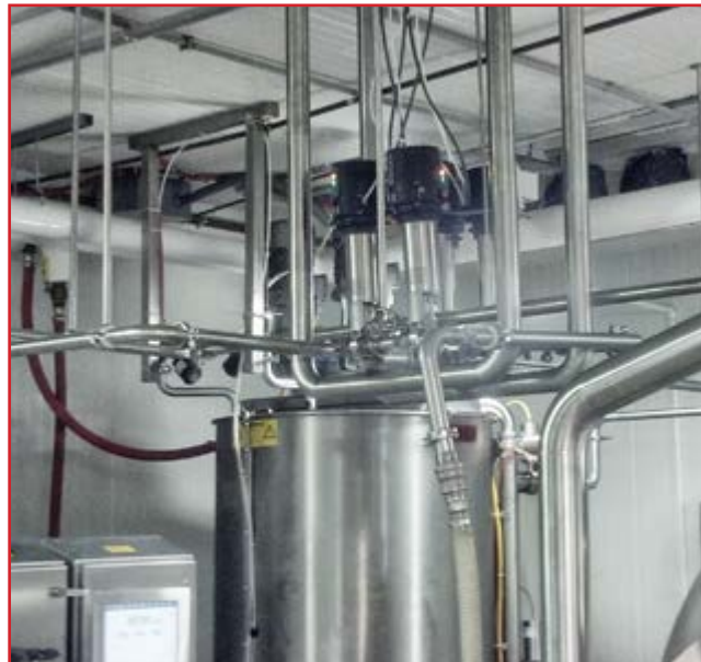
Valve Train for Multiple Liquid Ingredient Addition
